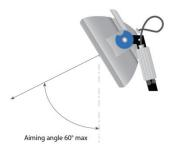
The lighting aiming angle (measured from downward vertical) shall ideally be  $\leq 60^{\circ}$  in order to minimise the glare to the players.
